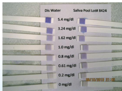
Figure 1. GPT-2 test strips response to glucose ranges in distilled water (left) and saliva (right).
